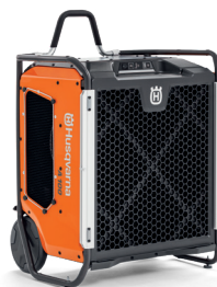
ALIMENTARE ELECTRICĂ HUSQVARNA A 45 0.5kW, 230V, monofazic, 2.3A, 1000m³/h, 20kg, IP54.
