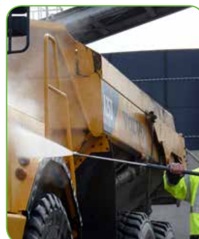
High pressure grit blasting lance with flat jet nozzle and suction hose, suitable for an operating pressure from \leq 350 bar and \leq 500 bar. code : 1.258.229.xxxxx
