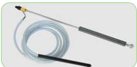
High pressure grit blasting lance with flat jet nozzle and suction hose suitable for an operating pressure from \leq 250 bar. Length : 900 mm code : 1.258.220.xxxxx
