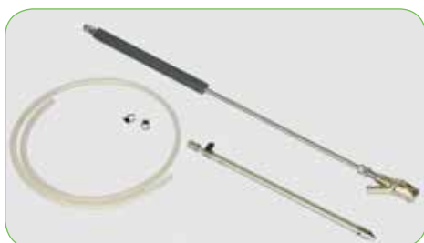
High pressure grit blasting lance with flat jet nozzle and suction hose, suitable for an operating pressure from \leq 350 bar and \leq 500 bar. code : 1.258.229.xxxxx
