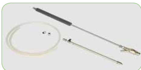
High pressure grit blasting lance with power jet hp nozzle and suction hose suitable, for an operating pressure from \leq 350 bar and \leq 500 bar. Length : 900 mm code : 1.258.225.xxxxx
